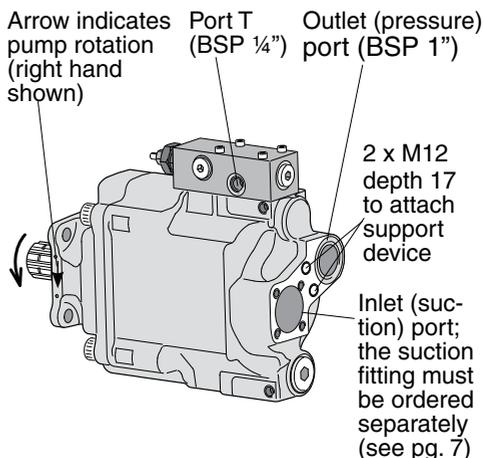
Fig. 1. VP1-095/-110/-130 main ports; right hand rotating pump.
